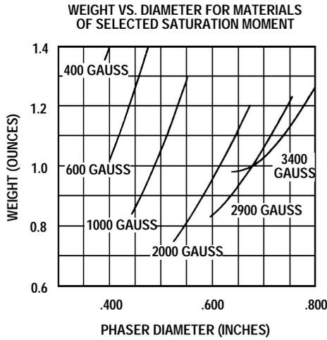
**Fig. 5:** Computed weight dependence on diameter for phase shifters using lithium-titanium ferrite
