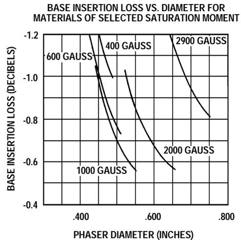
Fig. 4: Computed loss dependence on diameter for phase shifters using lithium-titanium ferrite.
