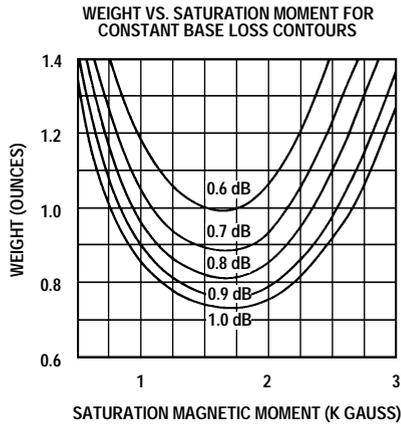
**Fig. 6:** Computed constant-loss contours of weight dependence on saturation moment.
