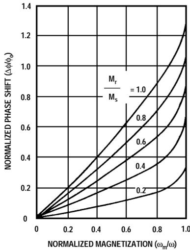
**Fig. 1:** Normalized phase shift for a circularly polarized plane wave in a remanently magnetized infinite ferrite medium.
