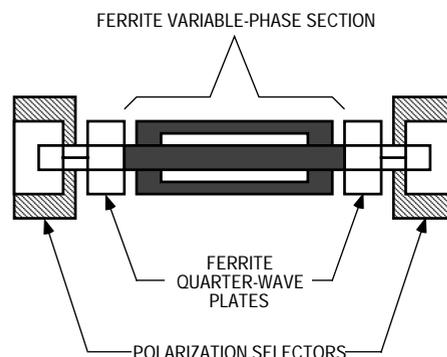
Fig. 2: Phase shifter configuration
