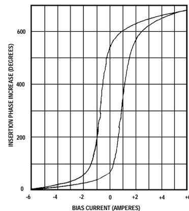
Fig. 6: Phase shift vs. current characteristic
